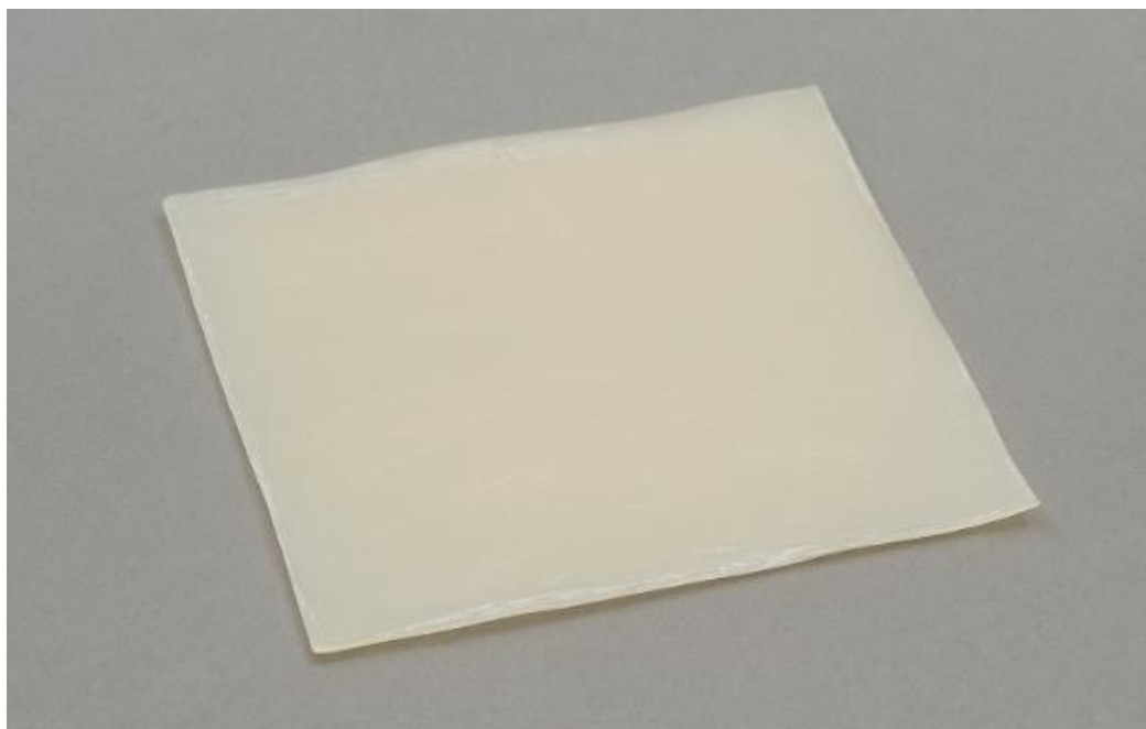
Fig. 4 Extracted PHA bioplastic film obtained after solvent evaporation.
